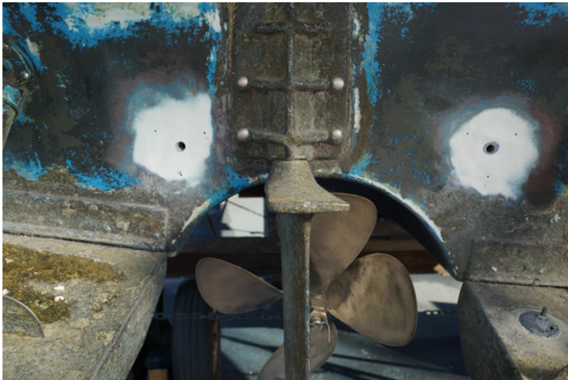
Sanded area and drilled holes. Ready for bottom paint
